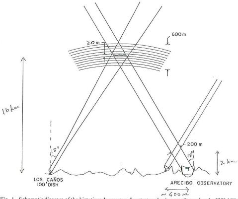
Fig. 1. Schematic diagram of the bistatic radar system for stratospheric sounding using the 2380-MHz at the Arecibo Observatory.
